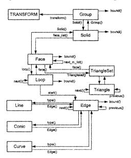
Fig. 3. Structure of the lightweight CAD file.
