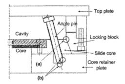
Fig. 1. Interference between two parts: (a) slide core and locking block, (b) angle pin and angle pin hole.
