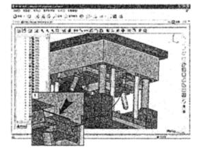
Fig. 13. Interference verification between the slide and lock.
