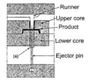
Fig. 2. Interference between the ejector pin and the core.
